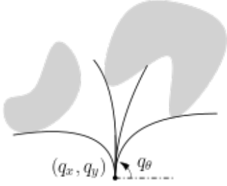
Fig. 4: A bendable touch sensor can be in multiple different modes at the same robot configuration. Therefore, the solution to the contact constraint is not unique.
