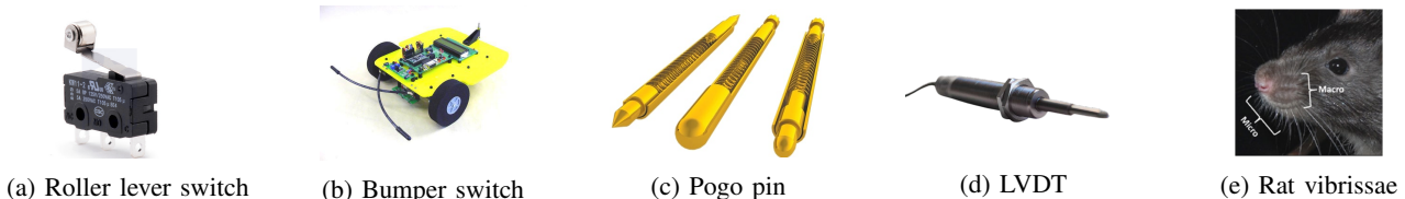
Fig. 1: Various types of touch sensors. 1a and 1b are common contact detectors; 1c and 1d are typical compressible touch sensors (Images from e-ptnk.co.kr/eng/pogo-pin/ and hoffmann-krippner.com/types-of-lvds/, respectively). LVDT stands for Linear Variable Differential Transducer; 1e shows macro- and microvibrissae in rats [1].
