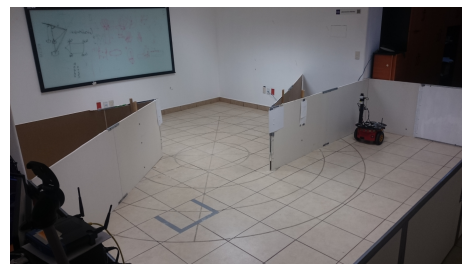
(a) Lab: This environment is a drywall made structure in the CIMAT robotics lab, it is composed of 6 straight line segments, 8 concave corners and 2 convex corners
