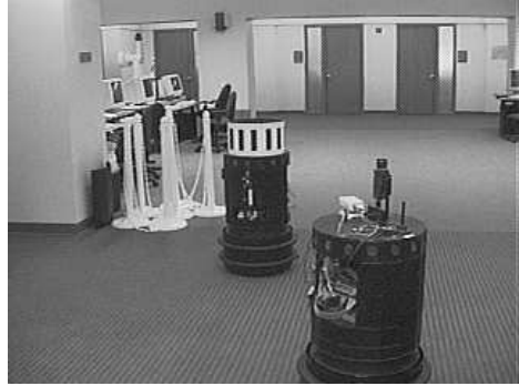
Figure 4. Two Nomad 200 robots are used for the experiments. One is equipped with a rotary camera.
