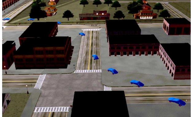
Figure 1: A designed trajectory for a car that drives through a virtual town at 72 kph. The vehicle dynamics are modeled as a nine-dimensional nonlinear systems that accounts for tire loading, skidding, and basic suspension effects.
