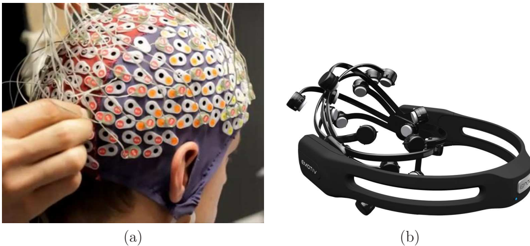
Figure 13.11: EEG systems place electrodes around the skull: (a) A skull cap that allows up to a few dozen signals to be measured (figure by Laboratory of Cognitive Neuroscience, EPFL, Switzerland). (b) Emotive wireless EEG device (figure by Emotiv and Emotiv EPOC+/Insight).
