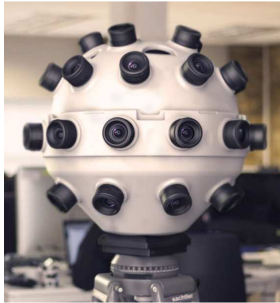
Figure 7.25: The Pantoptacam prototype from Figure Digital uses dozens of cameras to improve the ability to approximate more viewpoints so that stereo viewing and parallax from position changes can be simulated.
