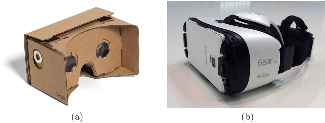
Figure 2.11: Two headsets that create a VR experience by dropping a smartphone into a case. (a) Google Cardboard works with a wide variety of smartphones. (b) Samsung Gear VR is optimized for one particular smartphone (in this case, the Samsung S6).
