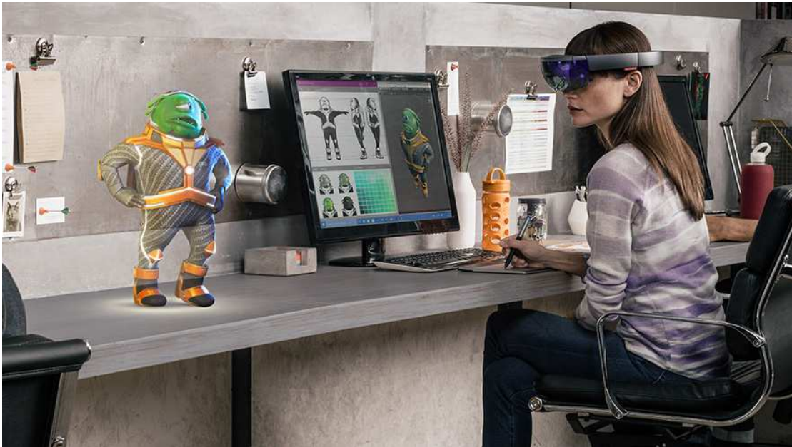
Figure 1.20: The Microsoft HoloLens, 2016, uses advanced see-through display technology to superimpose graphical images onto the ordinary physical world, as perceived by looking through the glasses.
